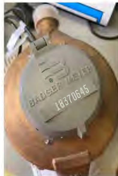
Photograph 3.13 Typical Water Meter
