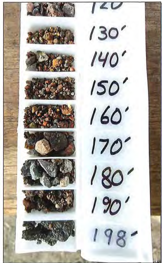
SHN characterized the subsurface material during the core drilling activities for Well 10.
